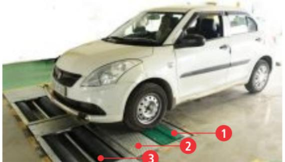
Test Lane equipment allows testing of passenger cars with a maximum weight of 3,500kg per axle. With the exclusive Test Lane Electronic Control and Modular Design, configuring your vehicle inspection line has never been easier, thus allowing you to choose the components best suited to your needs.
